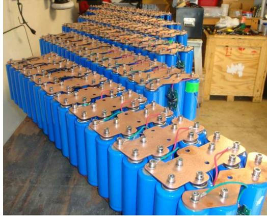
*Figure 3- Lithium Iron Phosphate Cells*
