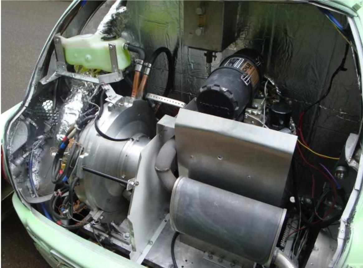
*Figure 2- POC Vehicle Generator System*
