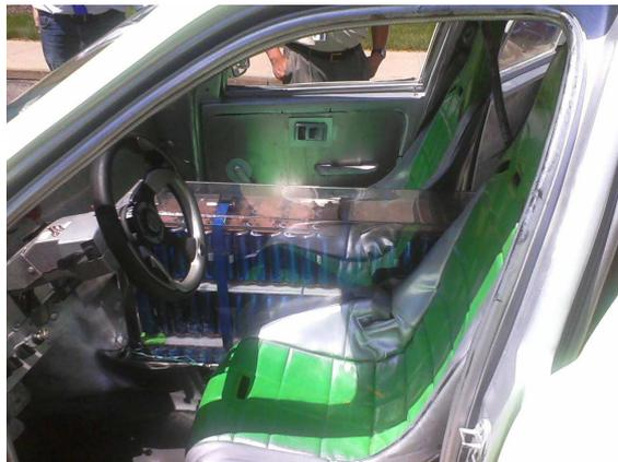
*Figure 4- POC Vehicle Battery Bank #1*
